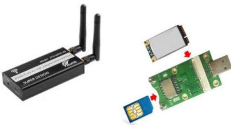
Unless one has plans to permanently install and use the modem within a laptop or PC, an external USB modem adapter is generally needed. There are a couple of inexpensive choices that most use (as shown in the photo with or without an enclosure.
